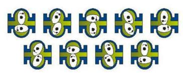
Each revolution the oval wheels displaces a discrete volume of liquid (defined by the space between the oval wheel and measurement chamber) through the chamber.
